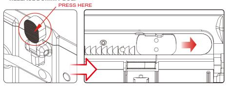
To Release bolt, just press the bolt catch.
