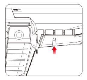
Press and hold the stock release button, then adjust the stock position.
