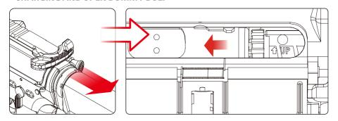
The charging handle can be pulled and the dummy bolt will lock and remain open.
