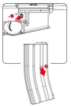
Press the magazine release button and pull the magazine downward to remove it.
